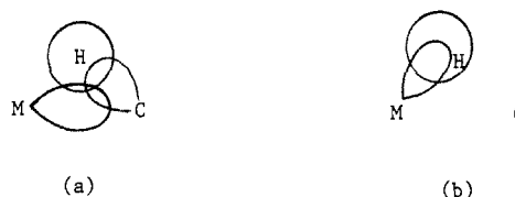
Figure 6. Possible bonding interactions between a C-H bond and a transition metal in a bridging C-H...M system. In what we have called the \sigma bond, an empty d orbital accepts electron density from the C-H bond by overlap with the H (1s) and C ( sp^3 ) orbitals (see a). In b, back-donation from a filled d orbital to the \sigma^* orbital of the C-H system is illustrated.
